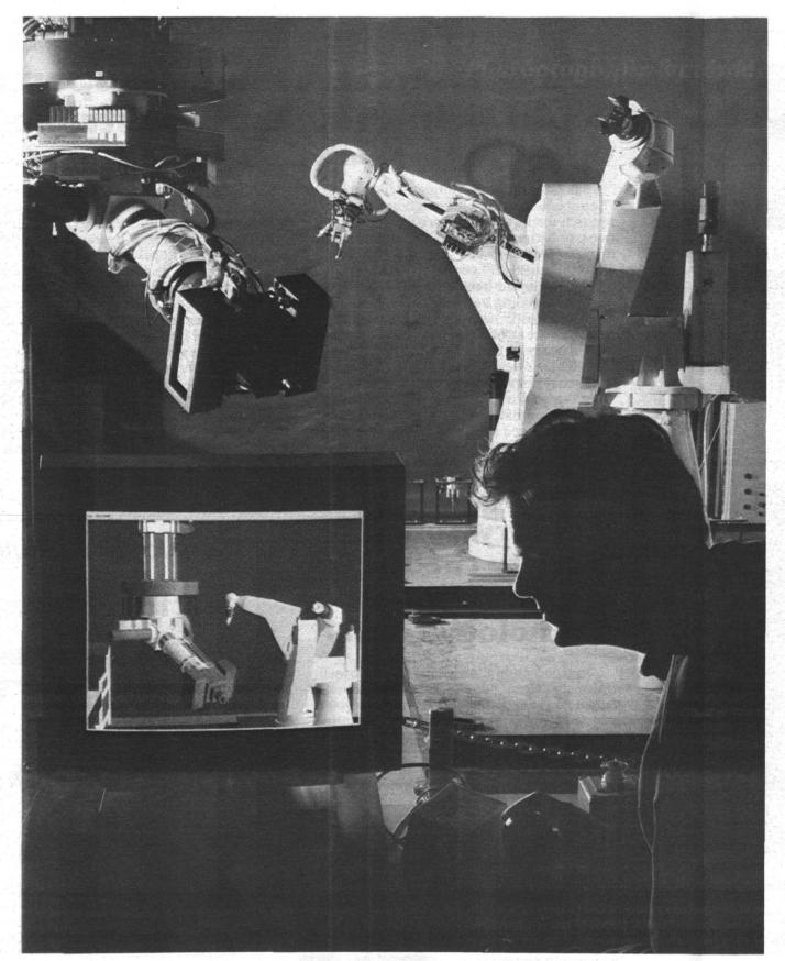
Michael McDonald (9661) programs three large manipulator robots in RMSEL's "megalab" with the help of Sandia's Sancho graphical programming system. Sancho allows operators to test robot motions on a computer, then download and execute the motions on actual robots. The system should help reduce the costs of integrating robots from multiple vendors on the production floor.
